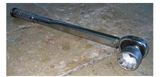
Use involves unlocking the micrometer type handle and turning it to line up the required torque setting on a micrometer marking or indicator window and then resetting the locking feature. The movement of the handle tightens an internal spring, which will cause a 'click' when the appropriate torque is applied by pulling the handle in a smooth arc toward you.
