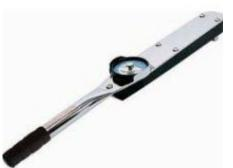
The dial type has a reaction indicator which moves around a dial indicating the torque applied. It is very similar to the beam type in that it requires observing the dial while torque is applied. Usually there is a witness needle adjusted against the indicator prior to the torque pull, which provides positive indication of maximum torque achieved.
