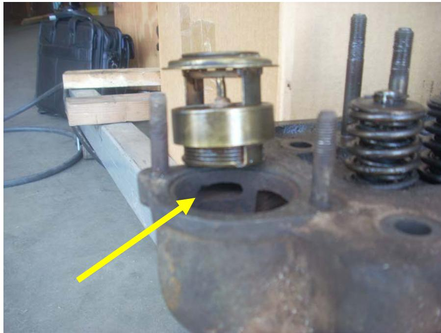
The six cylinder head bypass slot is identified in the picture above. The thermostat in the picture is designed for the bypass in that the shield moves up as the thermostat opens, moving the sleeve over the bypass opening. With the rise of coolant temperature, the wax in the actuating bellows starts expanding at 160° F fully opening by about 170.
