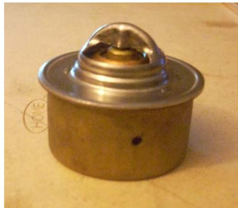
This \$15 bypass blanking sleeve on left is available from Moss Motors and other sources and it effectively closes the coolant bypass, improving cooling and provides a small restriction on the speed of the water flowing through the block and head reducing water pump cavitation.
