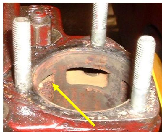
The A block Sprite engine is shown above left, identifying the external bypass hose and the function of the bypass flowing coolant from the head through the bypass hose, into the water pump and pushed back into the block by the water pump. The picture on the right shows the bypass slot.
