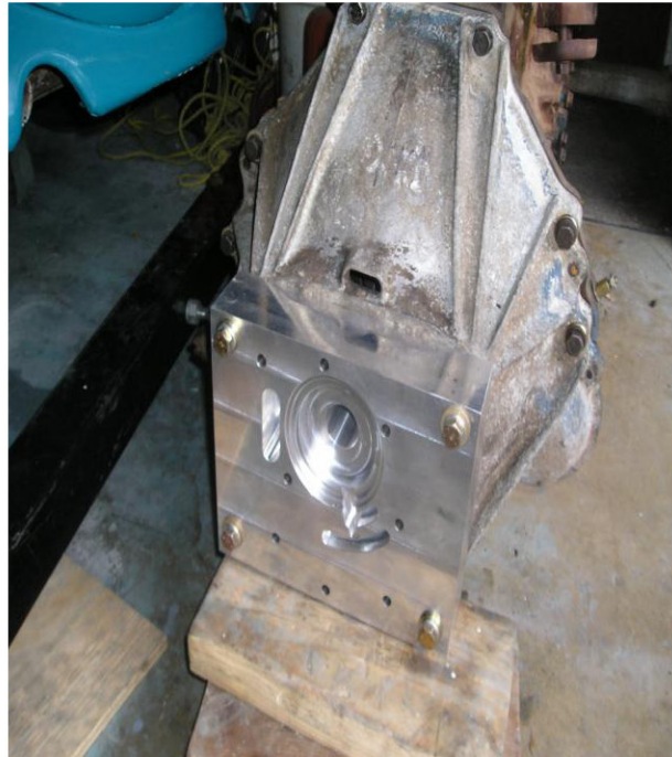
Too thick spacer plate bolted to the Maverick engine
