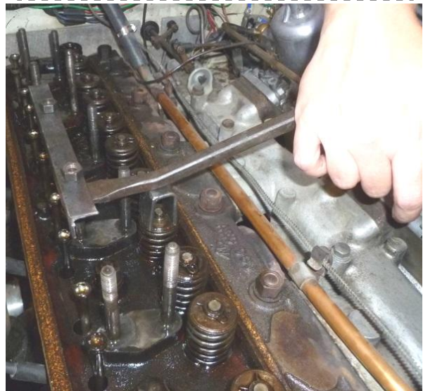
Home-made Spring Compressor
