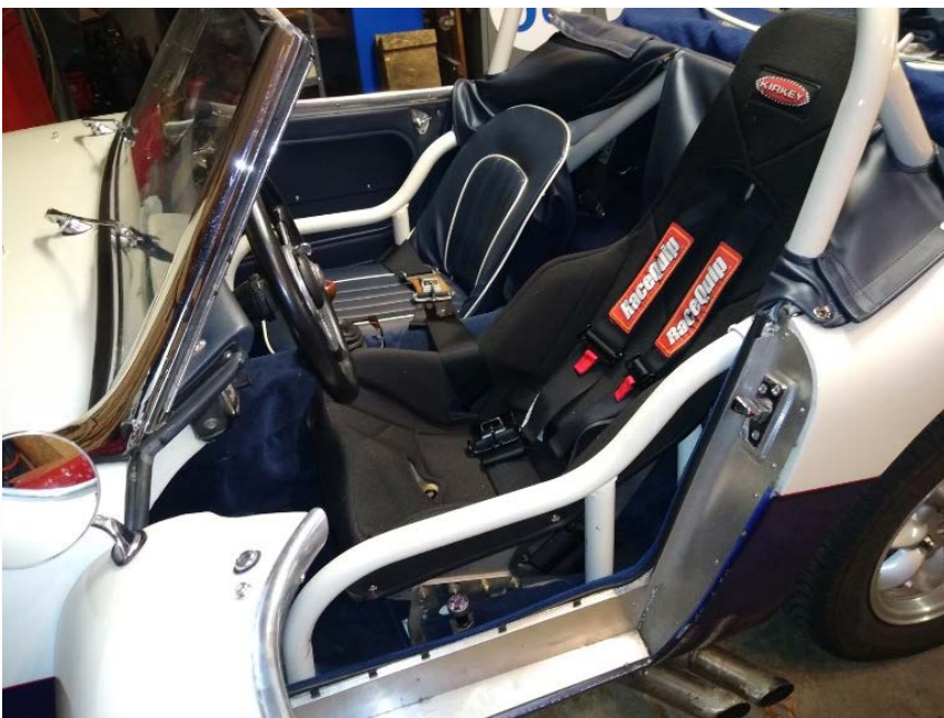
Interior picture showing the race seat and five-point Race harness, as well as the triangulation bars behind seats and the forward bars, which are removeable and bolt to the roll bar and structural angle welded to the outer sills and the front and rear outriggers.
