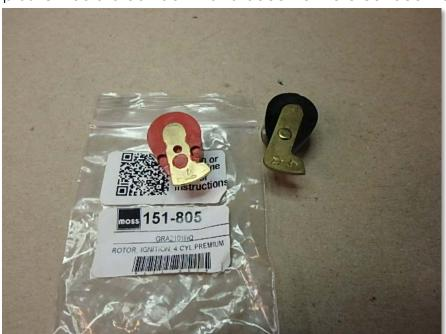
rivet would provide a path to ground on the rotor shaft.
